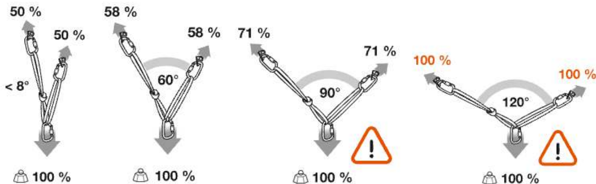
Magnification of vectors (Petzl)
